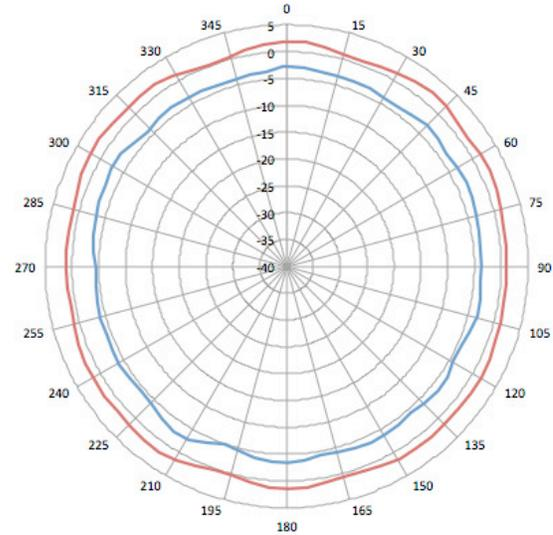
— 5.47GHz Average Azimuth — 5.47GHz Average Downtilt 30
